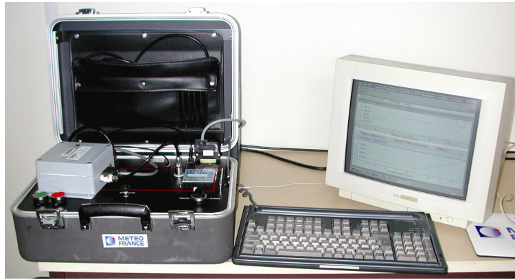
Photo 3: In situ pressure calibration system
