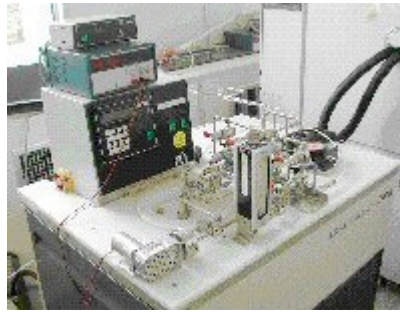
Photo 5: Generating bath of saturated air
